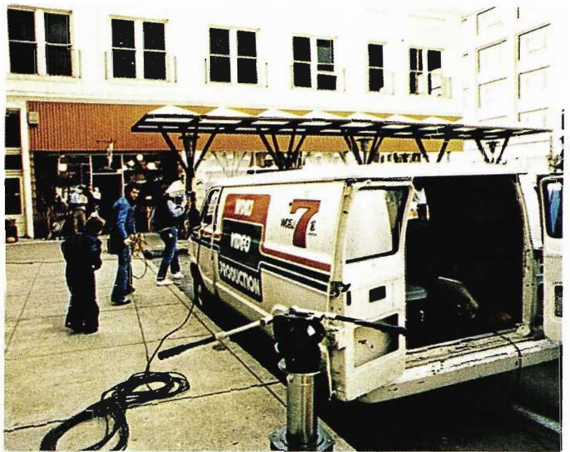
Location shoots involve the Ch. 7 production mobile unit; the self-contained rolling cart with 3/4-inch VTR and the TKP-45 camera.
