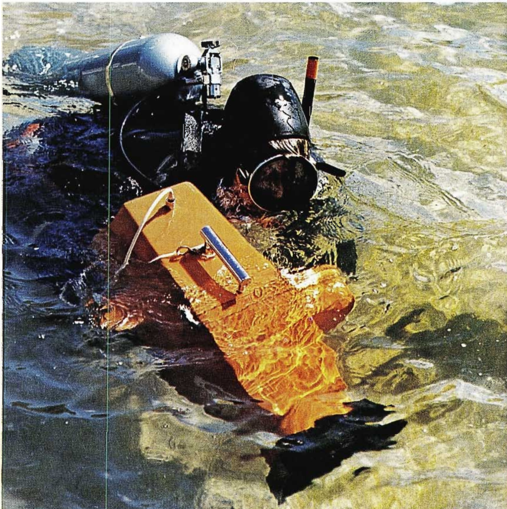
This sequence of photos shows the TK-76 camera with its special underwater housing designed by the technical staff of Channel TEN.
