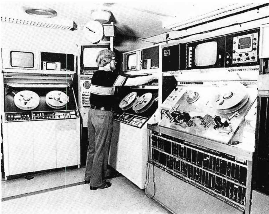
Video tape facilities include two TR-600A quad VTR's with AE-600 Time Code Editing systems. The editing system is being removed from the tape area to a separate editing suite.
