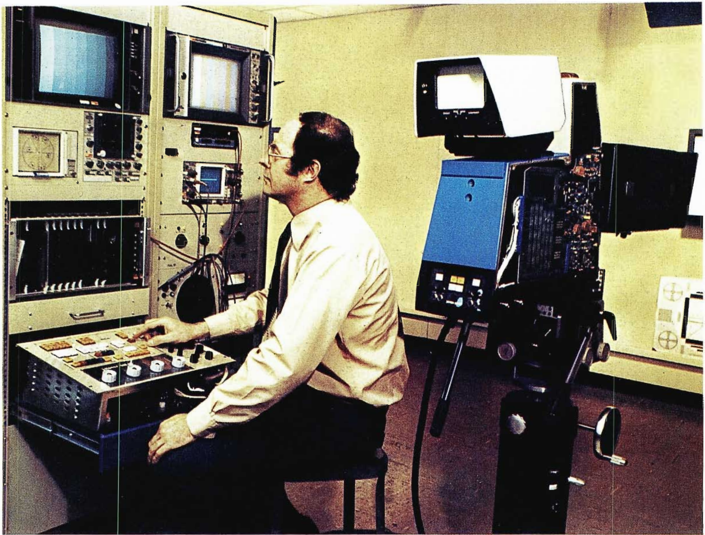
SYSTEMS TEST — A production model of RCA's TK-47 automatic color television studio and field camera is checked out by RCA engineer Frank Davenport during systems test in Camden, N.J. Introduced at the 1978 National Association of Broadcasters convention, the fully-automatic camera features simplicity of operation and microprocessor-
