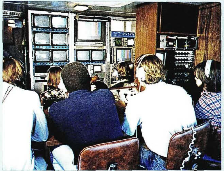
Interior of 29-foot mobile unit can accommodate as many as a dozen people. View from driver's seat shows audio and video switching; Director and AD positions in foreground.
