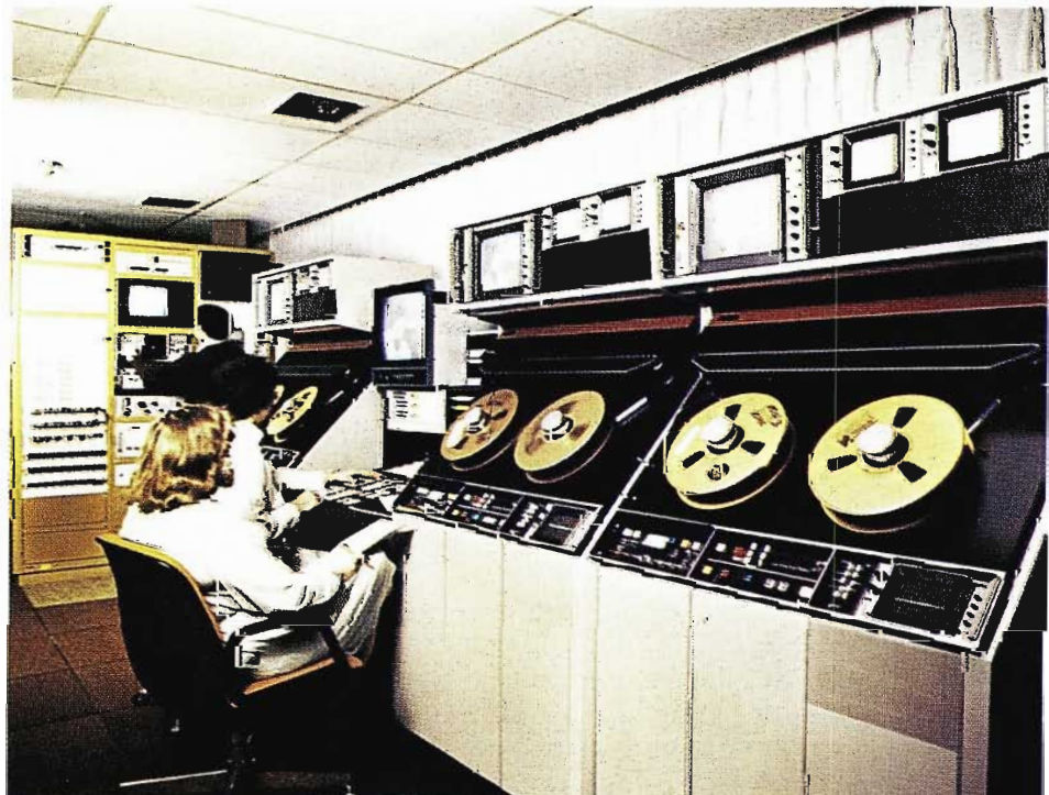
Quad tape editing system includes three TR-600A VTR's with AE-600 Time Code Editing System.
